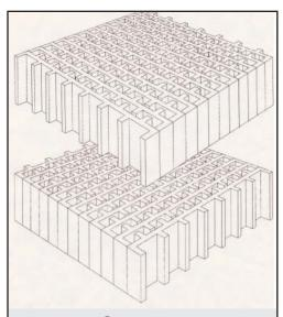
Figure 2. MLM<sup>®</sup> structured RTO heat recovery media from Lantec Products. Note that by rotating the plates of successive layers 90° that each successive layer is supported by the lower layer of media.
